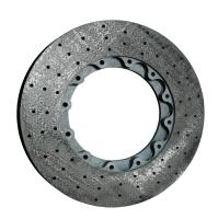
This carbon ceramic brake rotor has a special three dimensional carbon base which is made of long fibers. It is obtained through a proprietary process which gives the possibility of depositing a layer of material on both mating surfaces to improve the friction coefficient. The three dimensional carbon base provides higher strengths than the traditional short fiber bases and ensures more of a safety factor on tough extreme applications.
